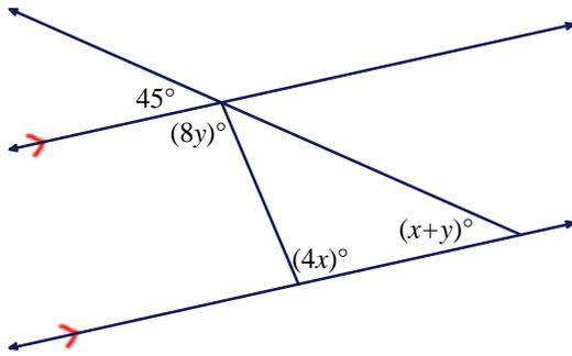
$$\begin{aligned} x+y &= 45 \\ 8y &= 4x \Rightarrow x=2y \end{aligned} \left. \vphantom{\begin{aligned} x+y &= 45 \\ 8y &= 4x \end{aligned}} \right\} \begin{array}{l} \text{Alternate} \\ \text{Interior } \angle\text{'s} \end{array}$$
